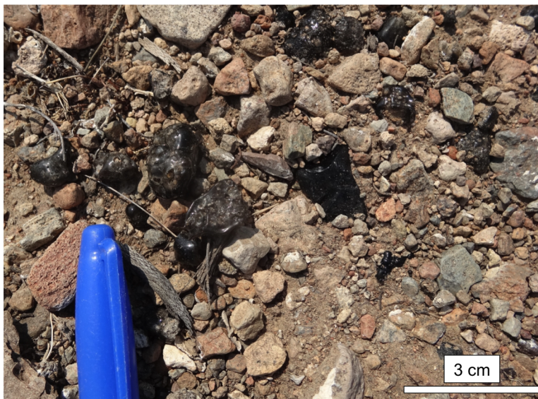
Figure 2.2: Photograph of typical sediment from near ground zero. The sediment includes fine clays and minerals as well as larger, centimeter-scale gravels and volcanic clasts. The dark, glossy objects visible in the image are fallout glasses. The blue object in the bottom left of the image is the cap of a Sharpie pen, shown for scale. In this image, irregularly-shaped fallout glasses tend to be larger than the more symmetric fallout glasses (such as those to the right of the pen cap).
